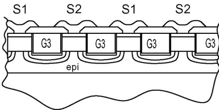
In the schematic, the shorting switch looks like two devices, two MOSFETs back to back, functionally, and it must block current in either direction when off. In the power IC, the shorting switch is implemented using single trenches with a common gate G3. The sources S1 and S2 are interdigitated alternately on opposite sides of adjacent trenches. No separate terminations
